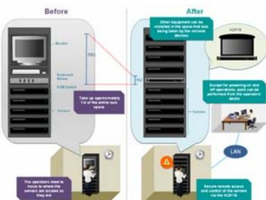
Adopting the KL9116 greatly benefited JSC by eliminating wasted rack space. In the past, a KVM switch and associated console devices ordinarily occupied almost 10U. Now, with the installed KL9116 taking up only 1U, JSC regains 9U of rack space that can be flexibly used for other devices.
